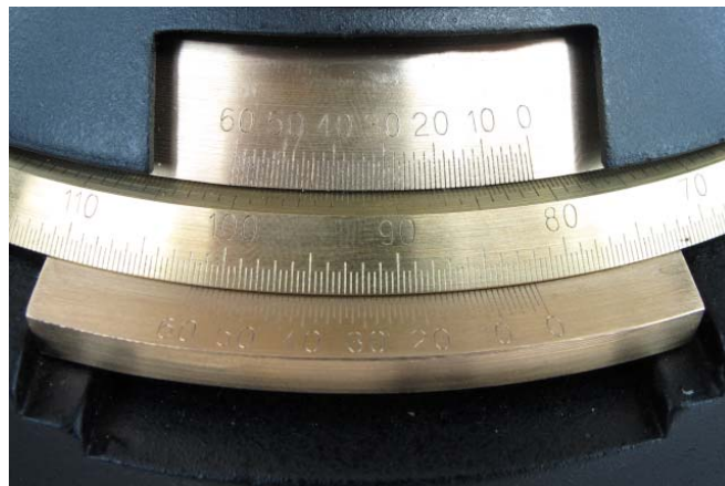
Fig. 3: Photograph of the angle scales: upper scale: position of the spectrometer table; middle scale: fixed with the collimator telescope; lower scale: fixed with the ocular telescope
