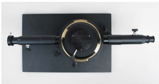
Fig. 6: Observation of the undeflected light
